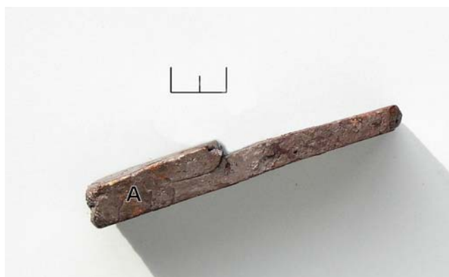
Fig. 2 Folded and forge welded piece Scale 1cm
