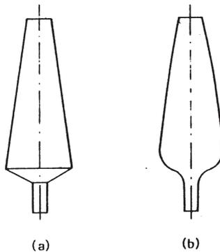
***Fig. 3: The original discontinuous Walloon shaft profile (a) and a more rounded (German) version (b)***
