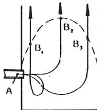
**Fig. 2: Blast flow pattern in a wide shaft**
