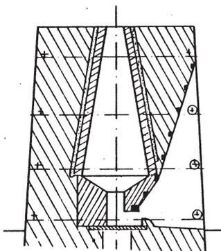
**Fig. 5: Section of a Walloon blast furnace**
