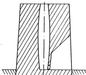
**Fig. 6: Section of a Brescian blast furnace**
