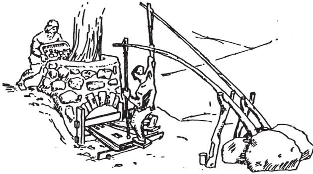
***Fig. 1: A reconstruction of a 13th century Trethütte in Noricum (Austria) (based on: W. Schuster; Das Alte Metall – und Eisenschmelzen; Dusseldorf; 1969)***
