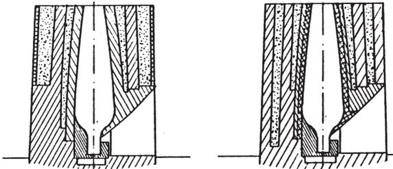
*Fig. 7: The German (left) and Walloon (right) blast furnaces in Sweden in 1650*
